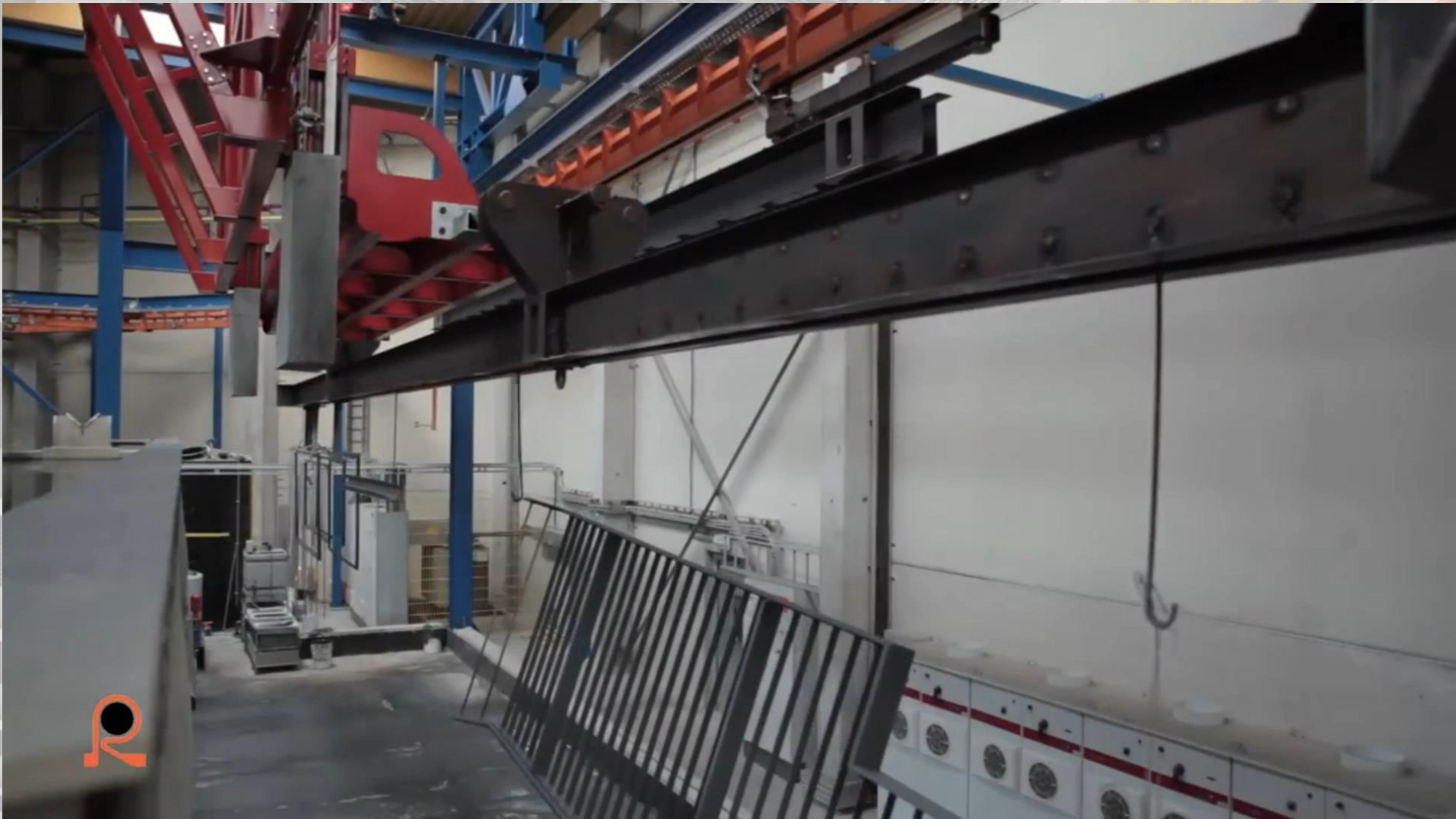
Transfer Of Flight Bar From Dip Pre-Treatment Crane Back To P&F Conveyor
